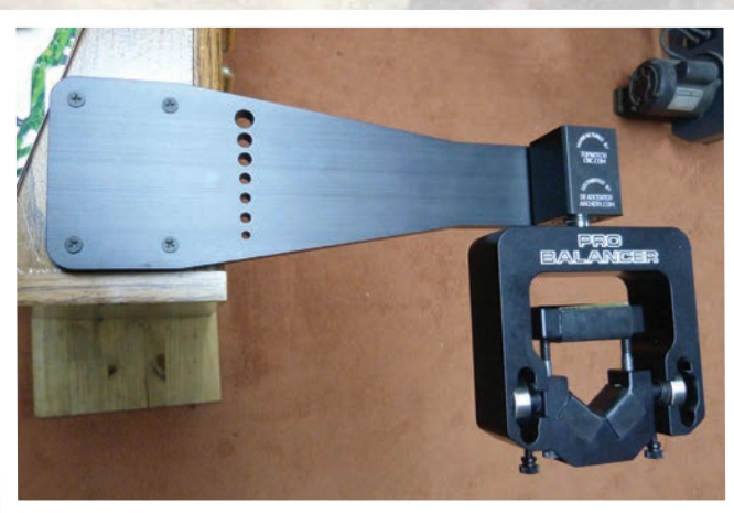
The Dead Center Archery Pro Balancer is a great way to get started with bow balancing. The device holds any bow at the grip section and allows it to pivot freely in two planes separately or in both simultaneously. The owner/inventor Todd Reich and I both like setting the left-right balance before setting the long rod tip-down balance. Fine tuning from long range will help you optimize the long rod tip weight to get the best groups.
